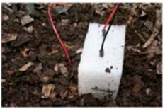
Dampness sensor will be utilized to discover vicinity of dampness at soil. We will embed this sensor into the dirt. It generally check the vicinity of dampness.
