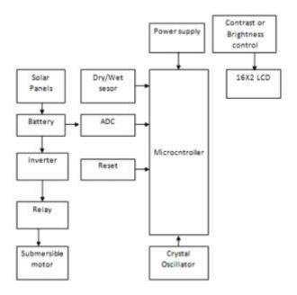
On the data side there are three sensors as demonstrated the structural engineering. Soil dampness sensor will check the dampness of the dirt according to the harvest which is to be developed. At the point when the dampness level of the dirt goes above or beneath the set worth, it will coordinate the microcontroller whether it ought to pump the water or not.
